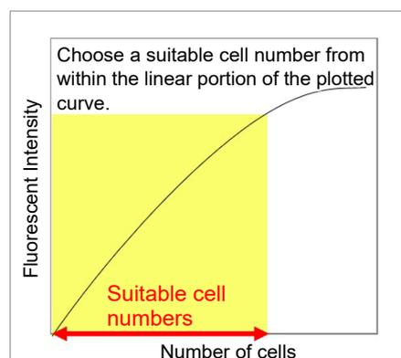
Plot the data on a graph, presenting the cell concentration on the x-axis and the fluorescent intensity on the y-axis. Then, the range of suitable cell numbers are indicated within the linear portion of the plotted curve.
