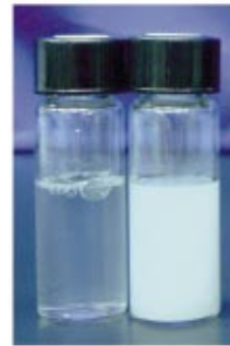
Fig. 2 Photographs of opaque emulsion and transparent solution of TMA-C2-DEA-C14 prepared by different methods.
